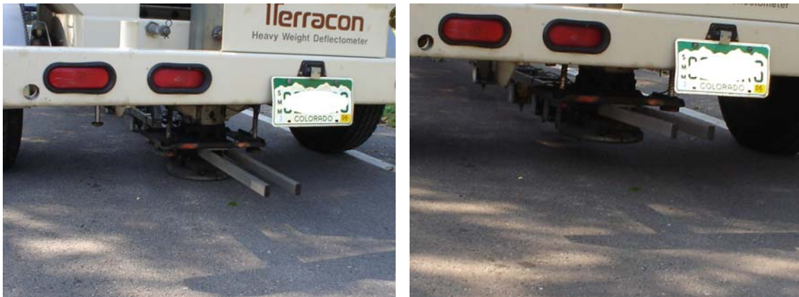
Figure 2. Picture showing circular plate for FWD load application and tips of dynamic displacement sensors.
